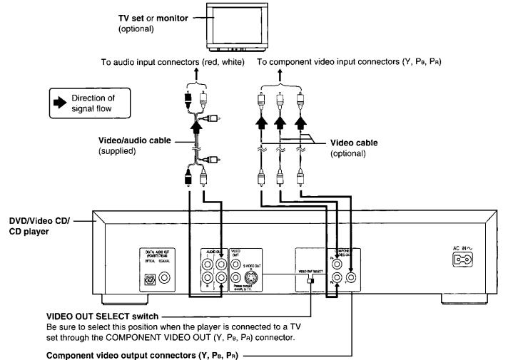
The component video output connector outputs the color difference signals (P<sub>B</sub>, P<sub>R</sub>) and luminance signal (Y) separately in order to achieve high fidelity in reproducing colors.
