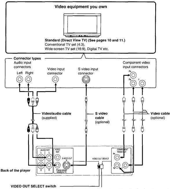
Select this position when the player is connected to a TV set through the VIDEO OUT connector or S VIDEO OUT connector. (The signal of COMPONENT VIDEO OUT is muted when you select this position.)
